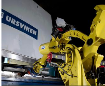
Robotic press handling system
